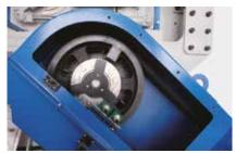
The internal high speed ram ensures optimal ingestion of lighter materials helping to achieve high outputs while requiring very little maintenance and reducing the risk of wear.
