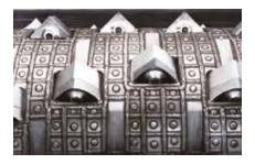
The ZERMA ZMS series shredders use large 80 mm concave ground square knives, producing high quality output. The cutters can be turned after a side is worn out.
